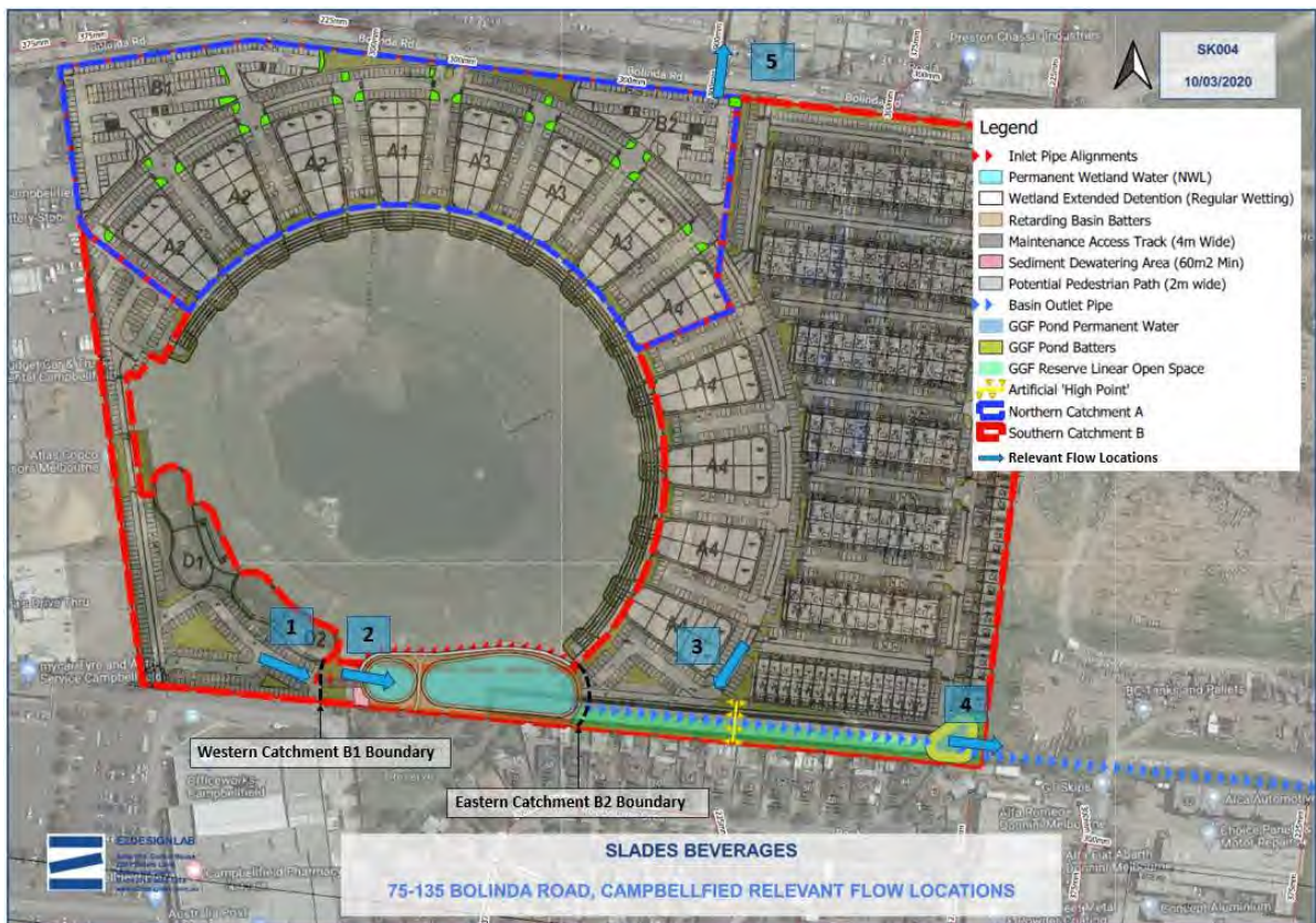
Figure 6 – Site catchment plan with relevant flow locations
