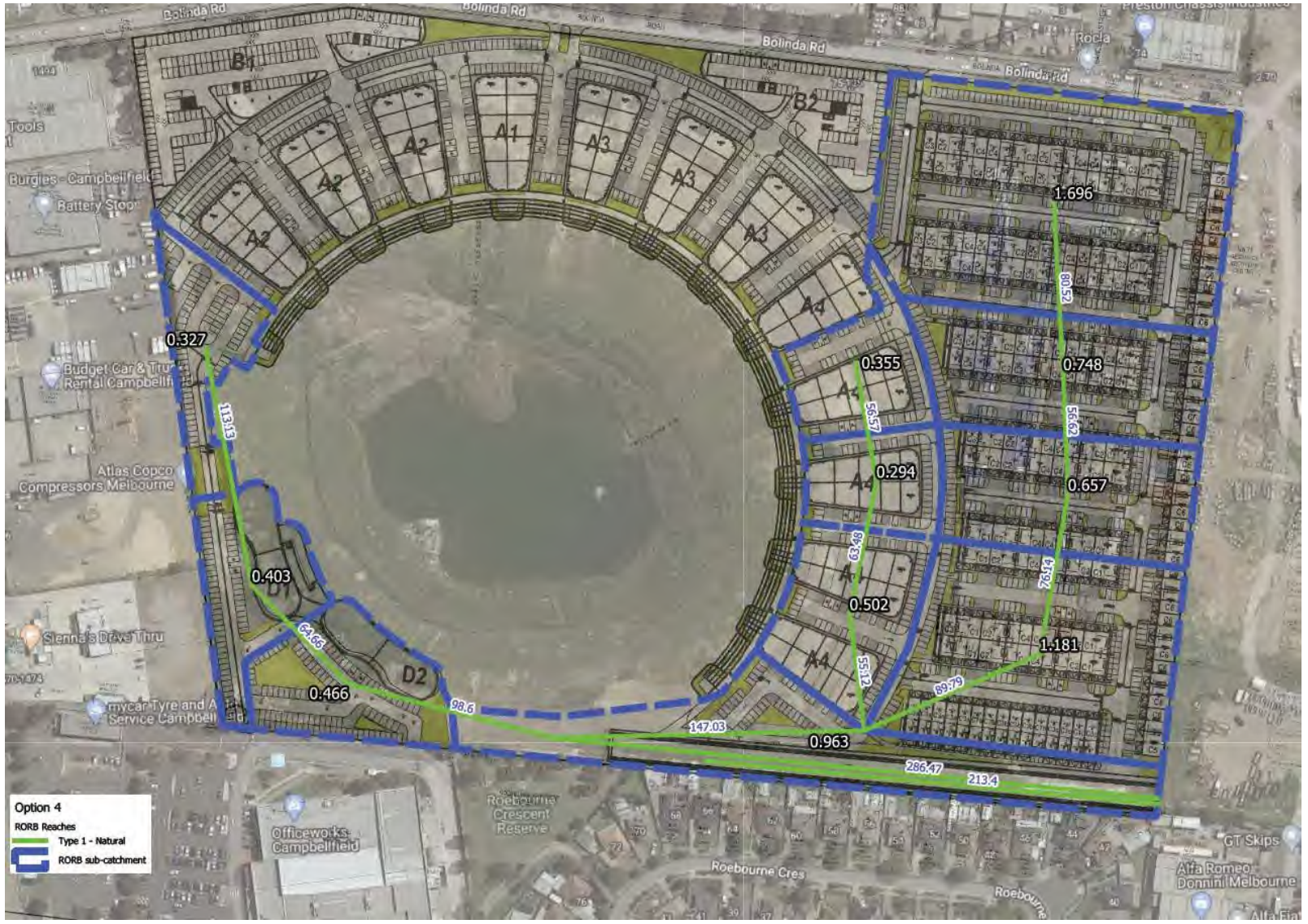
Figure 16 - RORB existing conditions catchment plan
